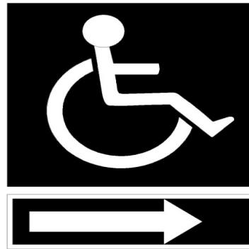
Figure 3.D.40 Accessible directional sign
